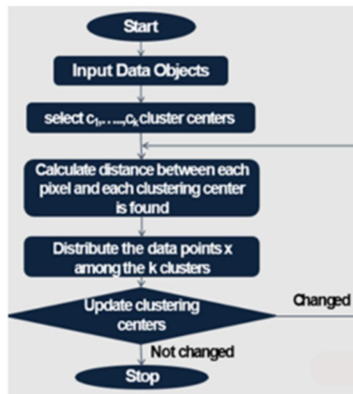
Figure 3. Data Flow of K means clustering algorithm
