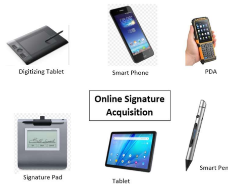
Figure 2. Various Acquisition Devices to capture online signatures
